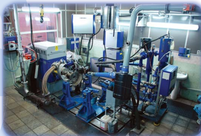
Test bench with automation system "PUMA", AVL, Austria
